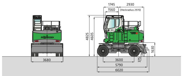
735 MHD with 1 m rigid forward-folding cab, undercarriage type MF37E
