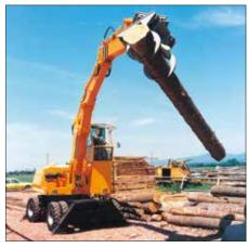
1974: Timber handling machine with elevated cab
